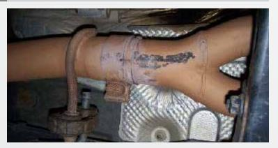
Loosen the clamp at the factory Y-Pipe. Remove the rubber grommets holding the exhaust. Loosen the connection at the head pipe and muffler, then remove the head pipe and let the muffler hang out of the way.
