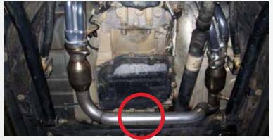
NOTE! The photo above shows the Y-Pipe as one piece. The Y-Pipe comes in 2 pieces and uses a supplied coupler. Install the Y-Pipe and only snug the hardware at the collectors and coupler. Re-install the cross member. Be sure to check the clearances around the Y-Pipe. Then tighten all the connections starting with the coupler, ensuring that both tubes are straight and aligned properly. Then tighten the collectors.
